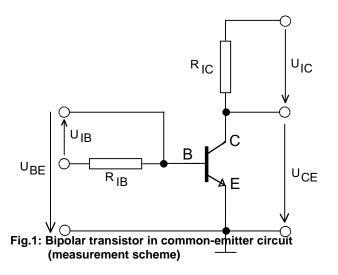
$$\begin{split} I_{C} &= f(U_{CE}) , U_{BE} = f(U_{CE}) \\ \text{at } I_{B} &= \text{const} \\ \text{and} \\ I_{C} &= f(I_{B}) , U_{BE} = f(I_{B}) \\ \text{at } U_{CE} &= \text{const} . \end{split}$$
